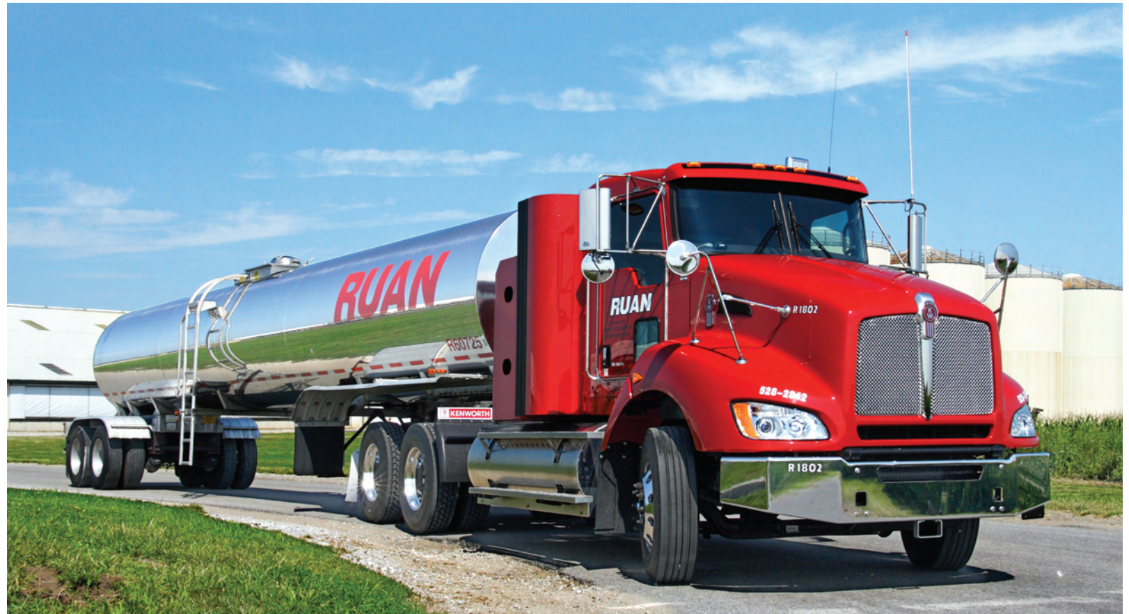
Operations are just getting under way for the new CNG-fueled milk hauling fleet at Fair Oaks Farms in Fair Oaks IN. With 42 Kenworth T440 tractors operated by Ruan Transportation Management Systems and leased from Paclease, it is being called the largest renewable CNG project in the United States. The operation also includes 80 milk tank trailers.
